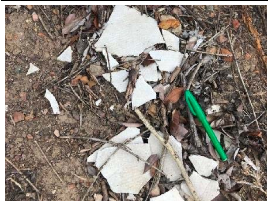
Image 6.10.1 View of fibrous cement sheeting fragments on the surface of the inferred fill embankment on the western side of the northern bowling green
